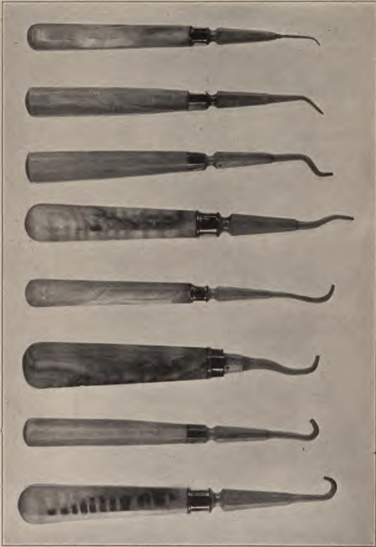
FIG. 33.—Ivory- and pearl-handled, gold-ferruled instruments for inserting gold fillings. Nos. 1 and 2 are awl-shaped for inserting gold and piercing center of pellet; the remainder are for condensing at different angles. (Author's collection.)
